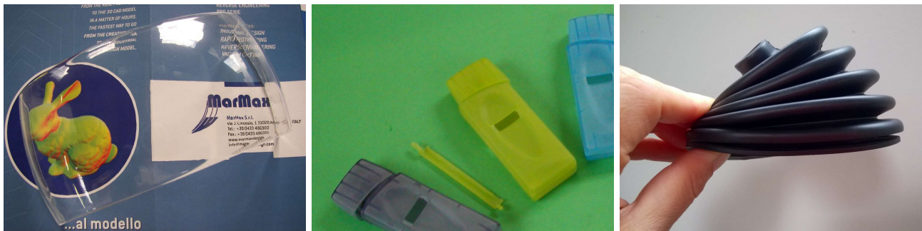
Picture 2: Transparent, elastomeric, translucent colored items, obtained from silicone molds.
